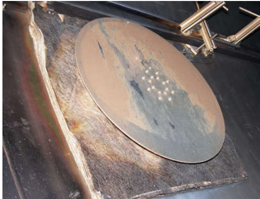
Figure 11. Cryopump cold plate after several weeks of thruster testing. Some of the deposits can easily be removed by wiping off with a cloth or with suction with a vacuum cleaner.
