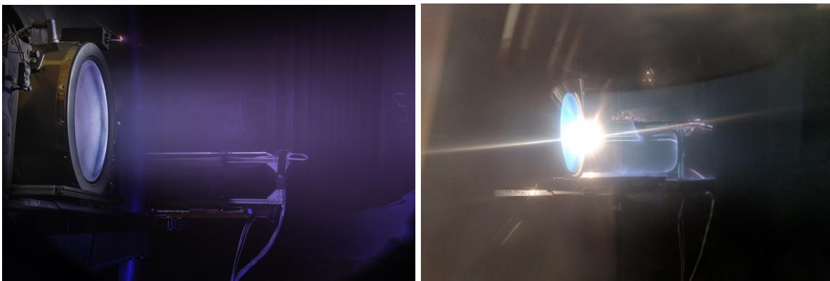
Figure 1: Photographs of probes in VF-16 next to the thruster.
