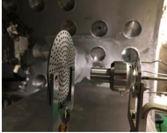
Figure 4. Hollow cathode experimental apparatus and the anode plate
