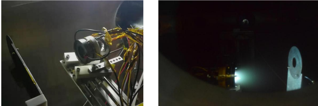
Figure 8. Left: ion thruster and thrust stand in the vacuum chamber. Right: plume of the thruster
