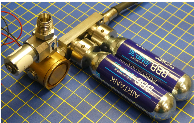
Figure 15. Prototype propellant subsystem with commercial off-the-shelf components: proportional valve, pressure regulator, pressure sensor and argon canisters.
