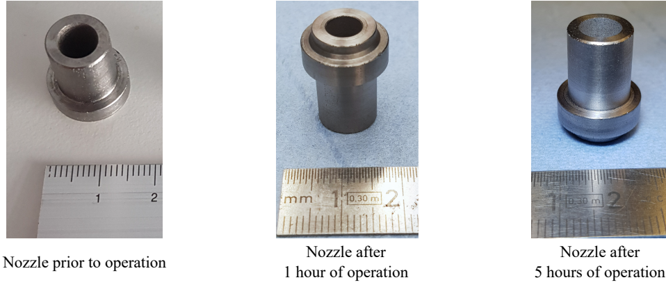
Figure 8: Nozzle outer surface prior and after thruster operation 11
