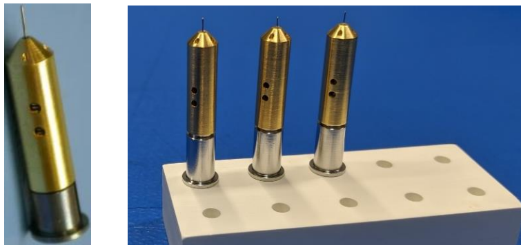
Figure 28. Capillary emitter fabricated for LPF (left) and emitters recently fabricated (right) to support future testing.
