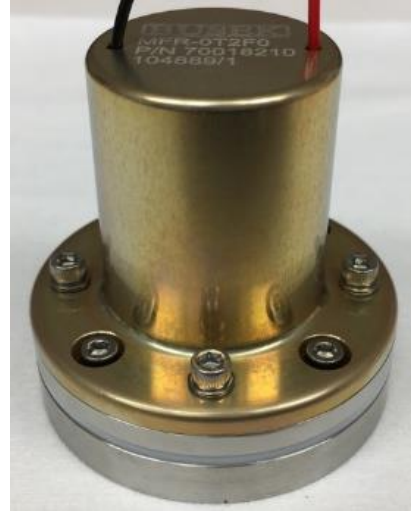
Figure 10. 4 th generation microvalve.
