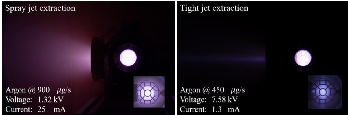
Figure 6. Operation condition of IEC plasma source with spray jet (left) and tight jet (right) extraction from D_c = 41.7 mm.
