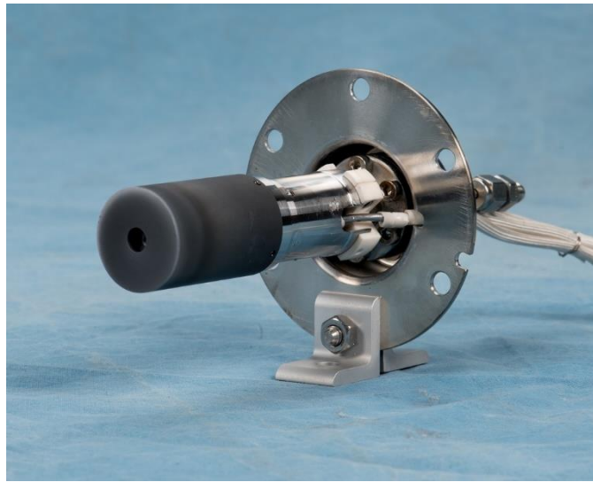
Figure 4. The Mark II cathode, a 25-A class barium oxide hollow cathode developed for the HERMeS Hall Thruster.
