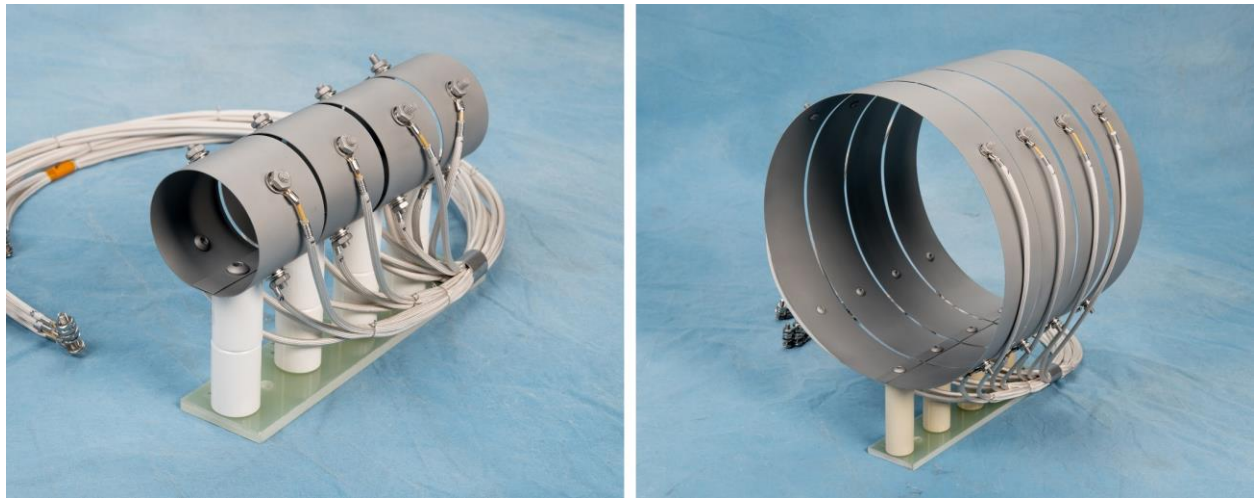
Figure 2. Photographs of the two molybdenum, axially-segmented anodes used in this experiment: the 64-mm diameter Small Anode (left) and the 254-mm diameter Large Anode (right).
