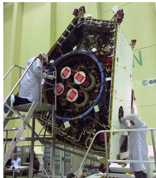
Figure 5. Electric Propulsion Thruster and Pointing Mechanism Configuration.
