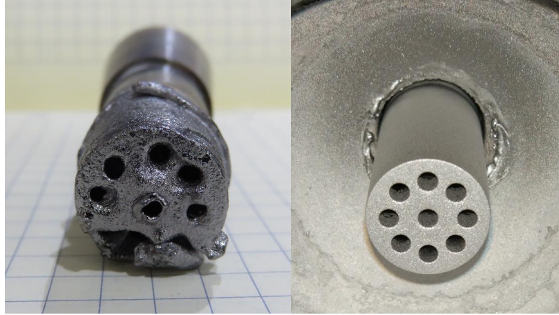
Figure 27 Cathode erosion characters
