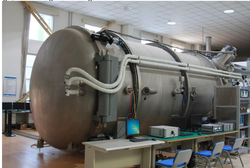
Figure 1 The vacuum chamber, employed in the experiment
