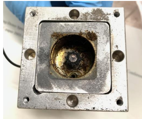
Fig. 11: Inside the discharge chamber after the experiment
