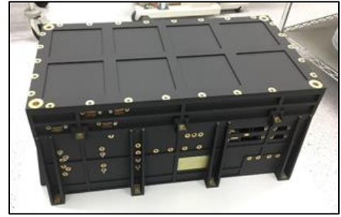
Figure 8 Mechanical Body of PPCU
