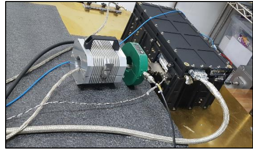
Figure 13 Conducted Type EMC Test Setup
