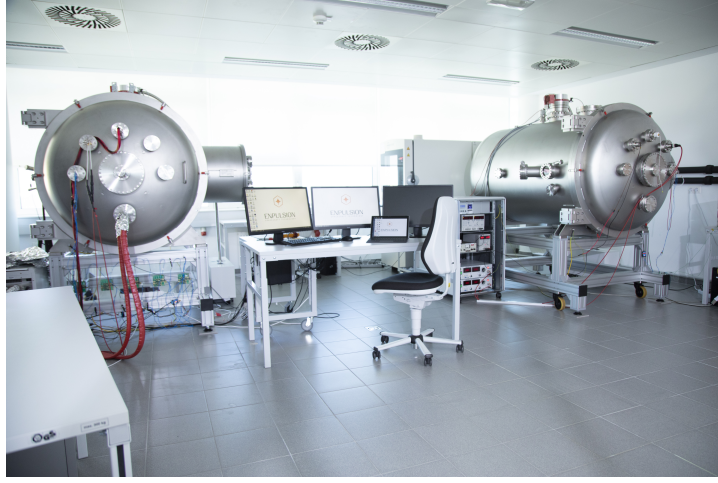
Figure 6: Vacuum chambers for acceptance testing
