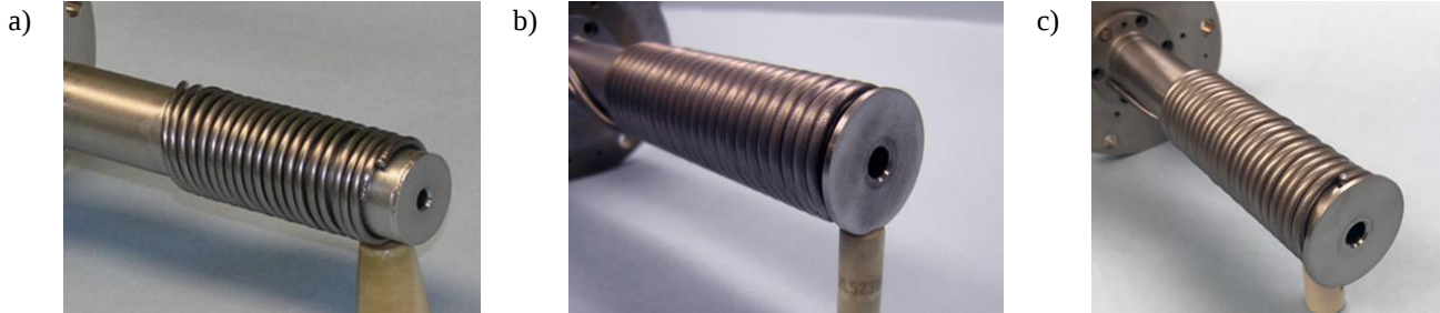
Figure 4 Original cathode orifice plate (a) and a versions (b) and (c) with a larger diameter orifice plates
