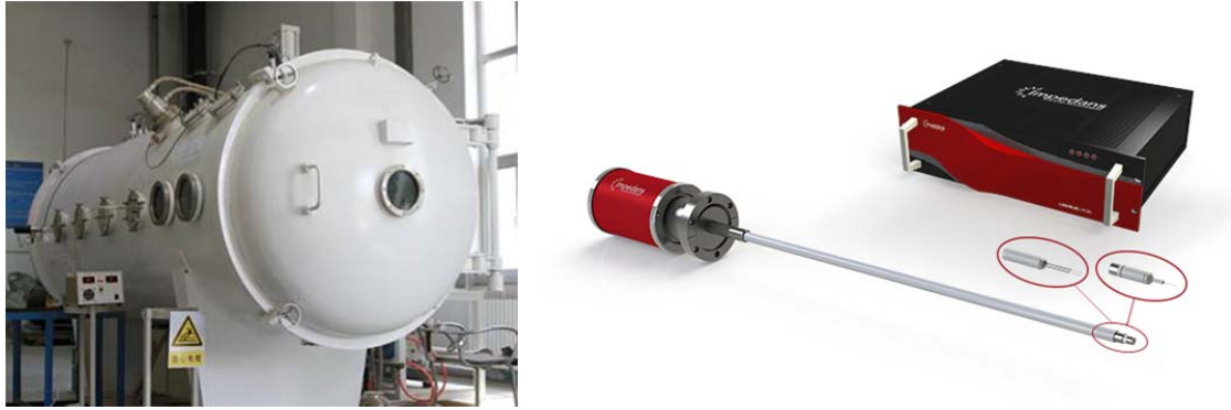
Figure 6. TS-6S vacuum chamber and Langmuir probe used in the experiment.
