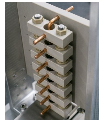
Figure 4: Electrical connections using RT liquid metal Galinstan
