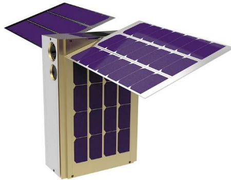
Figure 1: Illustration of a small satellite with deployable solar panels (NASA)
