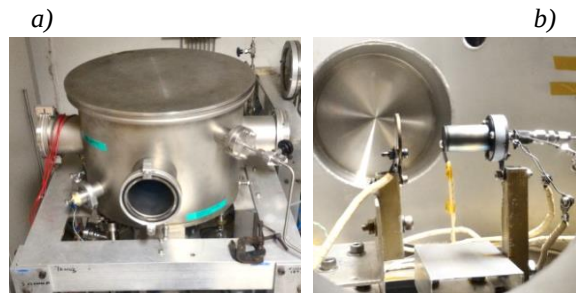
Figure 2. a) Cathode Experiment Vacuum Chamber (CEVAC) and b) PSAC cathode installed in CEVAC with the external anode (a K-type thermocouple is visible, touching the cathode's keeper electrode).
