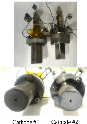
Figure 1. Low-current hollow cathode #1 and cathode #2 after experiments.
