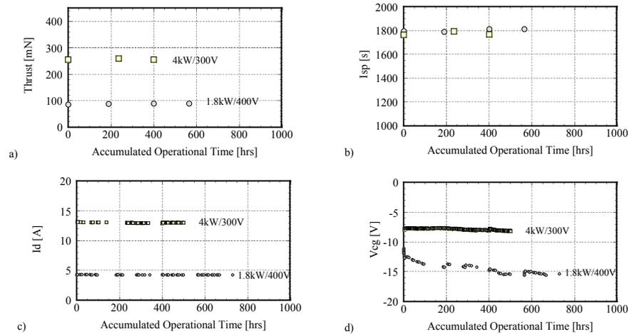
**Figure 10. Example Continuous Operation at Low Powers with BBM4 Thruster.**
