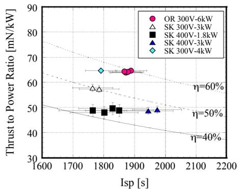
**Figure 8. Thruster Performance of BBM4 after 4,048 hours Operation at 6-kW.**
