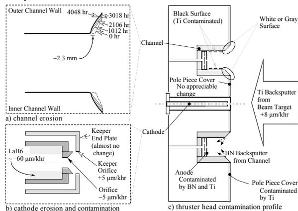
**Figure 9. Erosion and Contamination of 4,048hours BBM4 Thruster Operation.**
