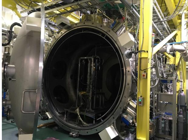
Figure 6. Hall Thruster Development Test (Hall-DT) Vacuum Chamber at JAXA.
