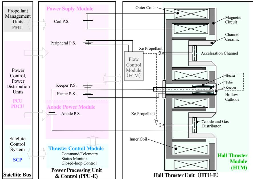
Figure 3. Schematics of Japanese Hall Thruster Subsystem.
