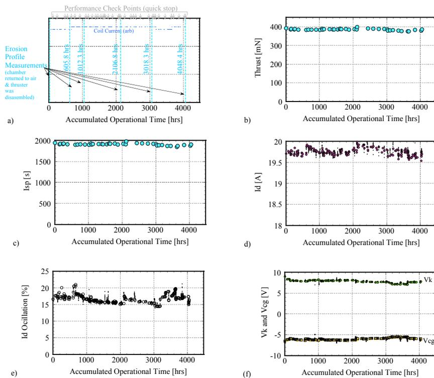
Figure 7. History of 4,048 hours Lifetest of BBM4 Thruster at 6 kW/300 V. a) event, b) thrust, c) Isp, (d) discharge current ( $I_d$ ), e)  $I_d$  oscillation, f) keeper voltage ( $V_k$ ) and cathode-to-ground voltage ( $V_{cg}$ ).
