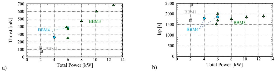
Figure 12. Performance of BBM-series Thrusters (BBM1a(100mm $\phi$ ), BBM4(150mm $\phi$ ), and BBM3(170mm $\phi$ ).
