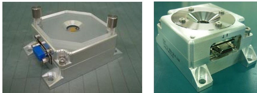
Fig. 6 Left: QCM installed on Hayabusa2 asteroid probe. Right: QCM for ETS-9.
