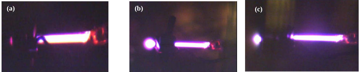
Figure 14. Photographs of a C 3 RFT with quartz capillary during operation in vacuum at 8 SCCM Ar: front electrode and biasing capacitor (a), back electrode and biasing capacitor (b), and short/no biasing capacitor (c). The plume in cases (b) and (c) is clearly visible outside the thruster.
