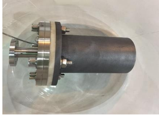
Figure 4 Lanthanum hexaboride hollow cathode assembly
