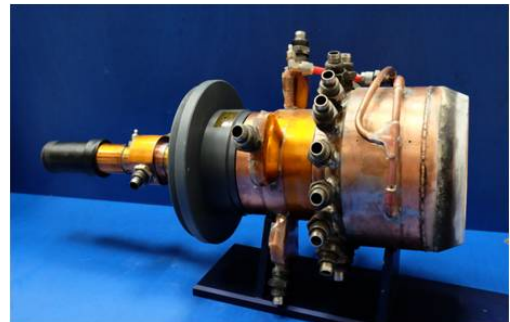
Figure 5. 100 kW thruster SX3. 4
