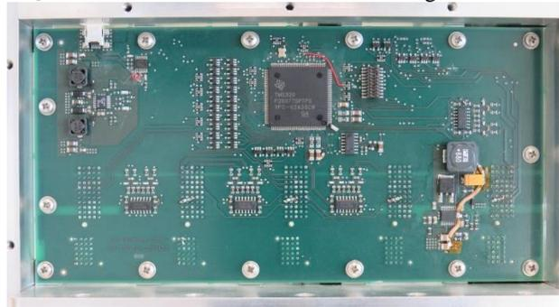
Figure 5: Backplane incl. Digital Control
