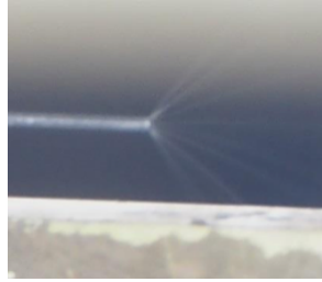
Figure 4. Irregular injection of ethanol from a capillary whose diameter is 100 \mu\text{m} .
