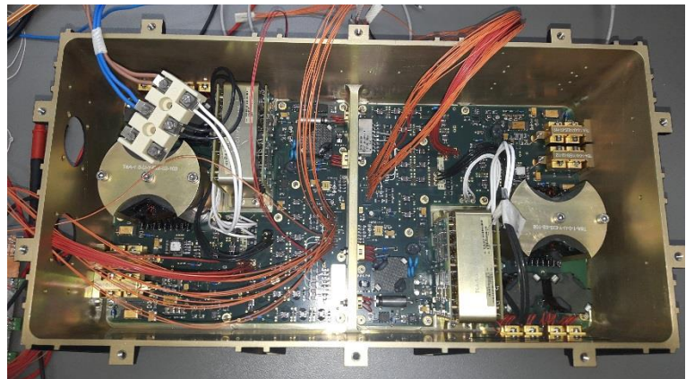
Figure 12. Primary and Redundant 1500W PPU in the case. Functional test after mounting.
