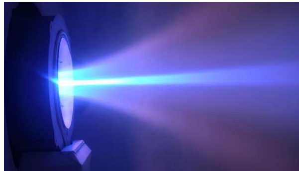
Figure 36. Argon plume with 50/50 mass flow rate distribution, 250 A, 157 V, 30 mg/s and 400 mT.
