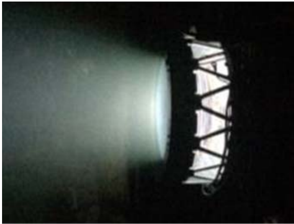
Figure 4 RIT 2X in operation
