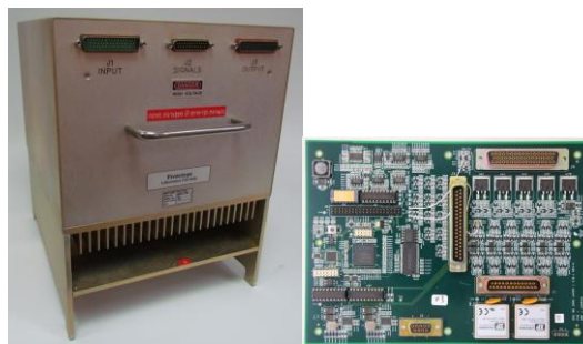
Figure 8. Picture of the R-400Mk2 PPU breadboard model and sequencer.
