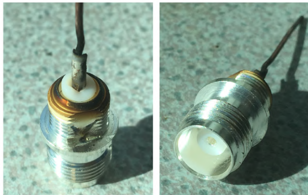
Figure 12: Pictures of the TNC connector damage sustained during the breadboard testing campaign.
