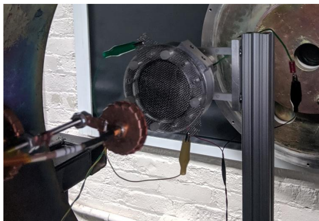
Figure 8. Image of the laboratory model of the gridded \mu CAT-MPS system inside the chamber.
