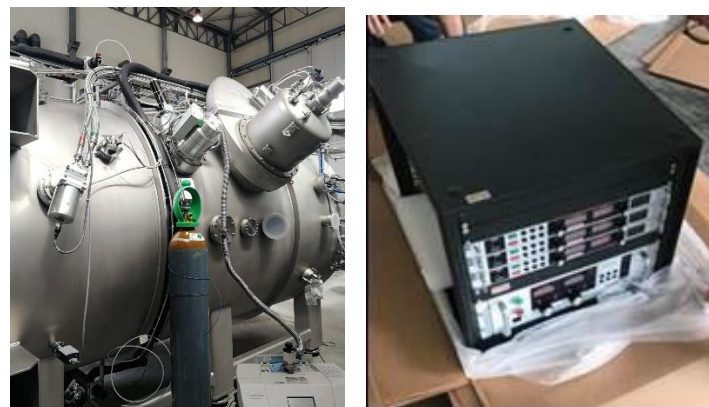
Figure 6. Lateral view of the simulator (on the left) and laboratory power supply rack (on the right).
