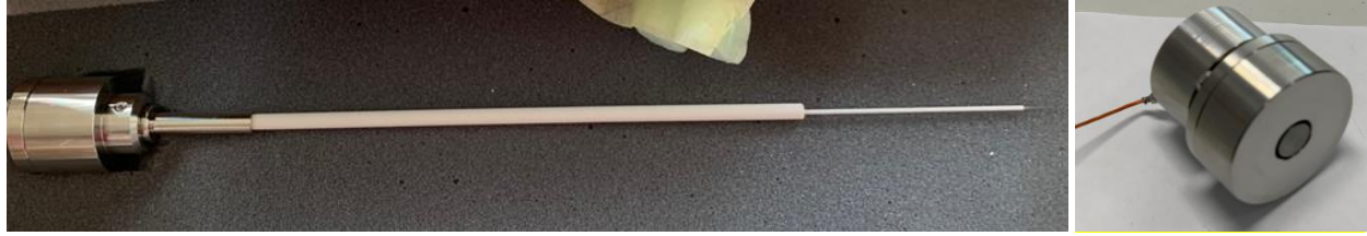
Figure 8. Intrusive diagnostics, equipping MSVC: a) Langmuir probe; b) Faraday probe.
