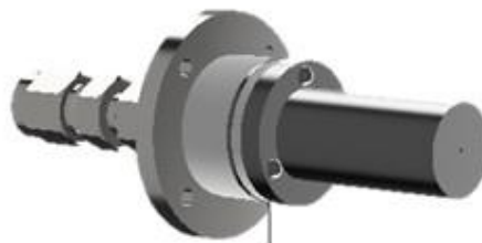
Figure 15. CIRA hollow cathode 3D model.
