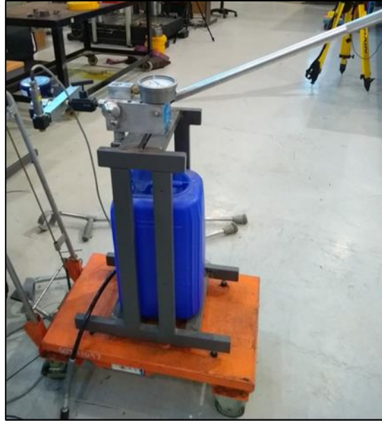
Figure 17 - Hydrapack hydraulic hand pump and manifold.
