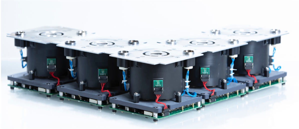
Figure 1. Several IFM Nano Thruster flight modules after acceptance testing
