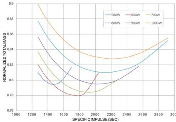
**Figure 4. Electric propulsion system sizing results for client vehicle orbit maintenance only.**
