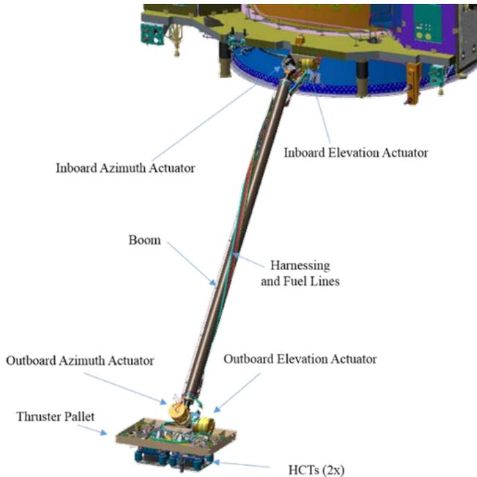
**Figure 8. Thruster Pointing Assembly on MEV-1.**
