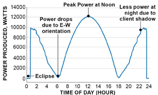
Figure 3. Power during equinox season for solar arrays oriented in E-W direction on servicing vehicle.
