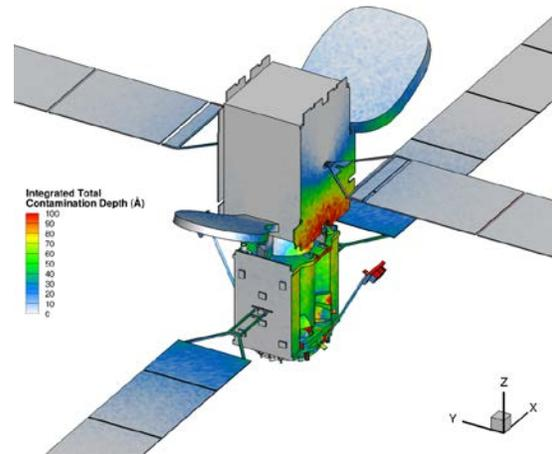
Figure 5. Integrated MEV/Client Vehicle plume compatibility analysis.
