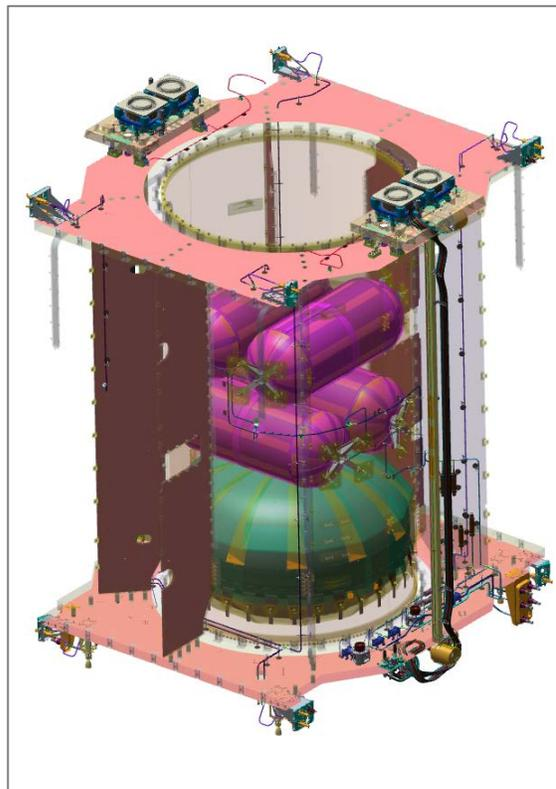
**Figure 6. MEV hybrid monopropellant chemical and electric propulsion system.**
