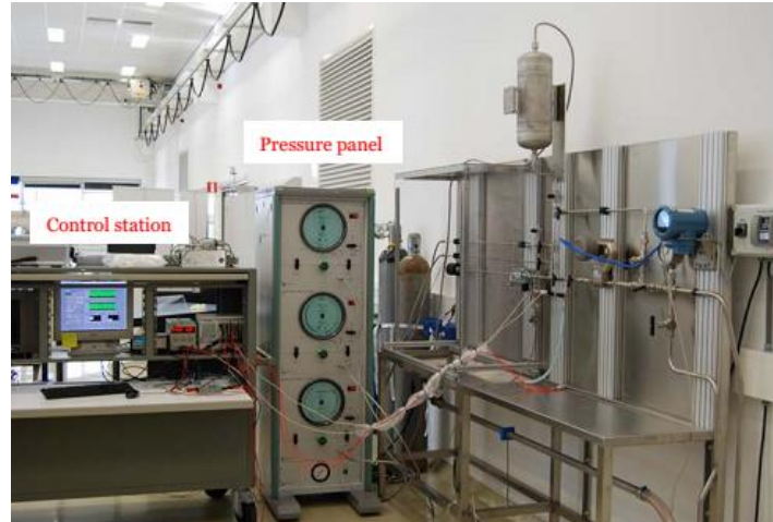
Figure 3. EPL Flow Rig Bench
