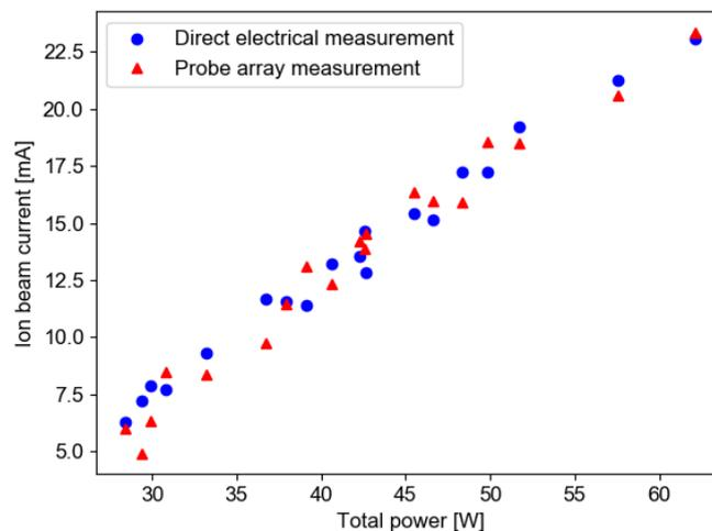
**Figure 4 – Ion beam current over all studied operational modes, showing the comparison between the direct electrical measurements and the estimation from measurements performed by the probe array.**
