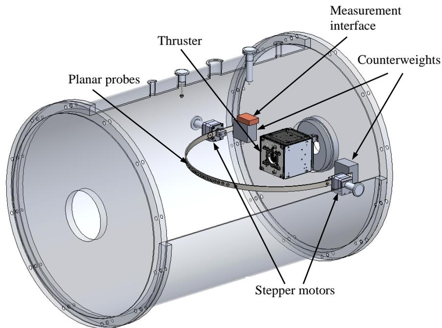
**Figure 2 – Instrument construction and positioning inside the vacuum chamber.**
