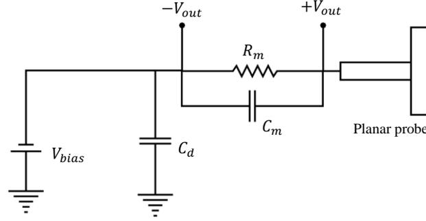
Figure 1 – Planar probe measurement circuit.
