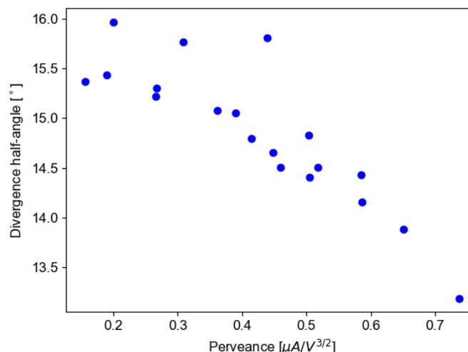
**Figure 5 – Divergence half-angle dependence on perveance for all studied operational modes.**
