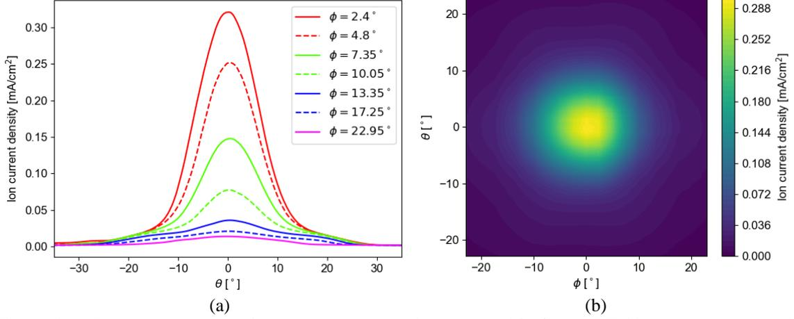
**Figure 3 – Measurement by the instrument at operational mode 18 of the NPT-30, presented as the (a) signal measured by 8 channels of the array, (b) the reconstructed bidimensional map.**
