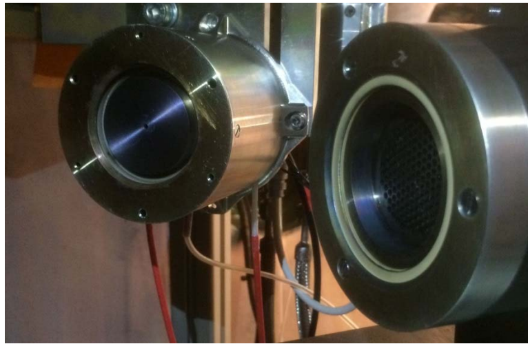
Figure 9 Coupled test - RIT-μN (left) and RIT-μX (right)
