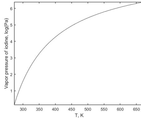
Figure 1: Vapor pressure of iodine as a function of the temperature in logarithmic scale
