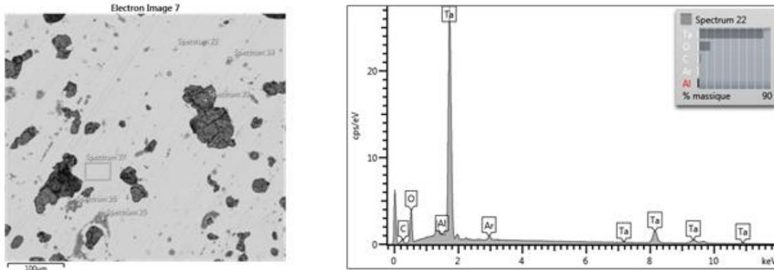
**Figure 5: X-ray micrograph analysis of an Al7075-T6 alloy coated with Ta2O5**
