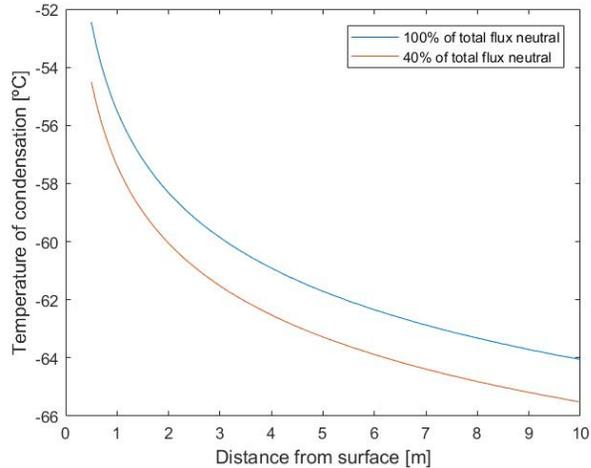
**Figure 3: Temperature of condensation of neutrals for a gridded ion thruster as a function of the distance from the exit plane**
