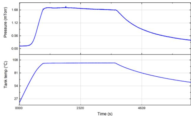
**Figure 9: Pressure at the chamber and temperature of the tank for a firing**
