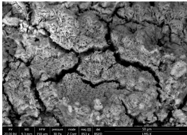
**Figure 4: Aluminium 6082 micrography, BSED detector, 853x**
