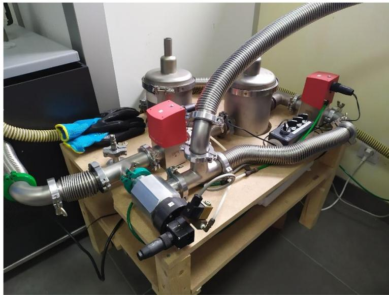
**Figure 8: Cold trap system for the testing of the NPT30-I2**
