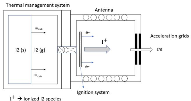
Figure 2: Schematics of the NPT30 ion thruster
