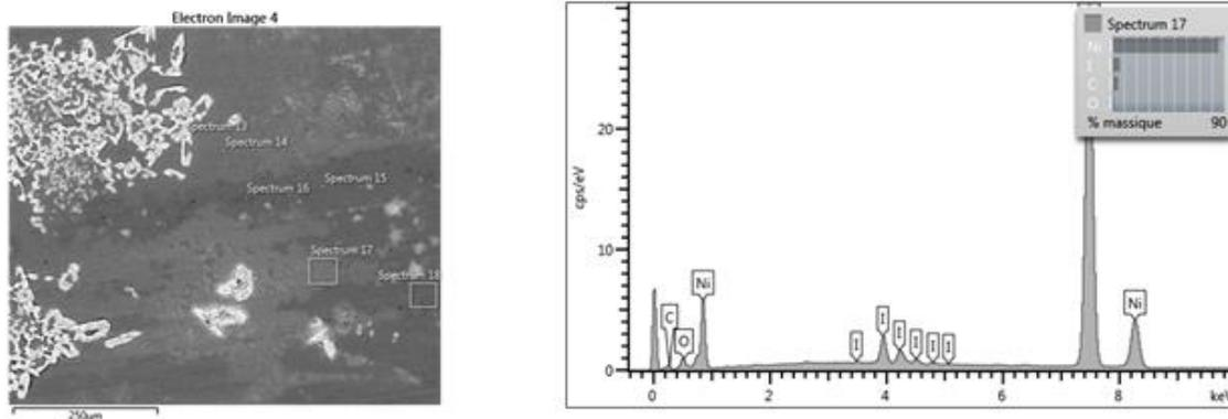
**Figure 6: X-ray micrograph of a nickel sample**
