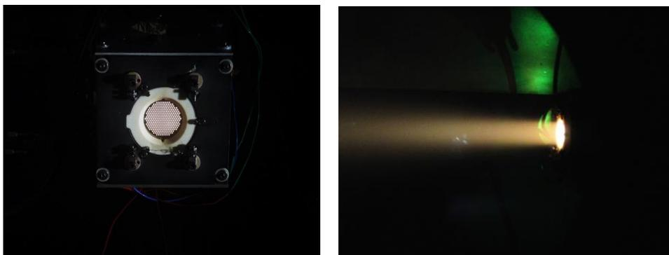
**Figure 11: View on the NPT30-I2 propulsion module during plasma ignition (left) and beam acceleration (right) tests.**
