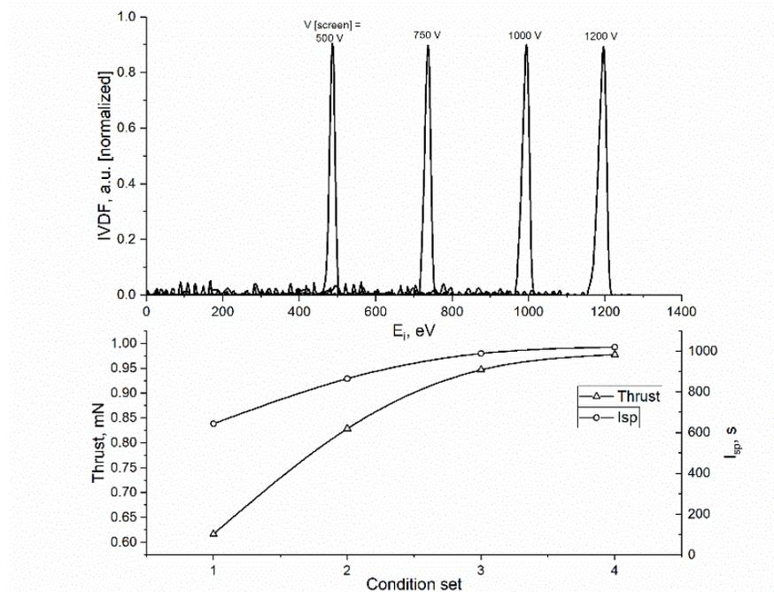
**Figure 12: Ion velocity distribution functions (top) and thrust/specific impulse (bottom) for the NPT30-I2 thruster prototype. acceleration (right) tests.**
