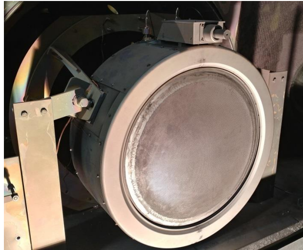
Figure 1. Dev-C engine mounted in the vacuum facility prior to pump down.
