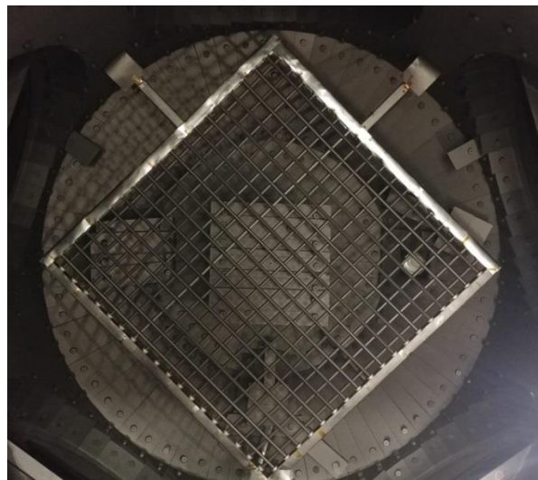
Figure 7. Far-field probe assembly used for characterizing the thrust vector.
