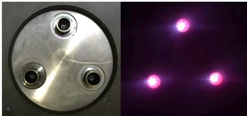
Figure 4. Photograph of MPD cluster system on the wall of the chamber (left: out of operation, right: MPD cluster in operation)
