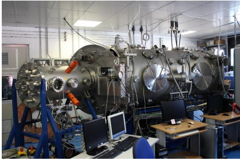
Figure 2. SITAEL LFF vacuum facility.
