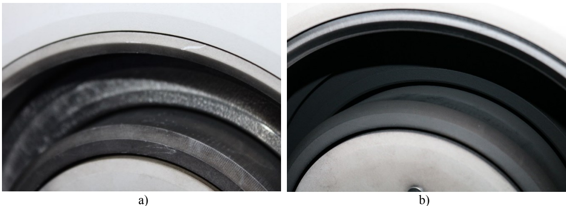
Figure 24. Detail of the HT5k DM3 ceramic channel before (a) and after (b) the test campaign.
