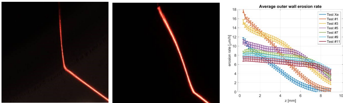
Figure 7. Outer channel wall profile at the beginning of the tests (left) and at the end of the campaign (middle). Average erosion rate measurement at multiple points of the endurance test (right).
