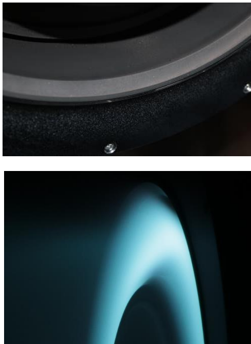
Figure 7 Graphite deposition on the ceramic channel after the characterization test (top), and detail of the plasma detachment from the channel walls.
