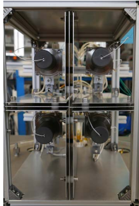
Figure 5. Qualification heater test setup
