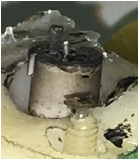
Figure 8. a) The lifetime-end 10 hz passive mode. b) A new set of cathodes for a passive mode run
