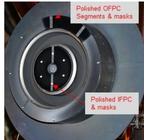
Figure 18. Pole cover configuration for the B2 segment of the MS Optimization Test.
