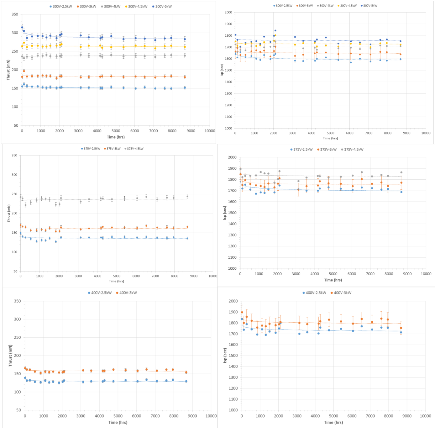
Figure 12. EQM1 performance characterization measurements during the life test. Left: thrust; right: I_{sp} . From top to bottom: data at 300 V; 375 V and 400 V of discharge voltage.
