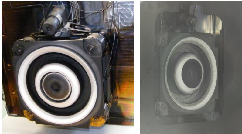
Figure 4. PPS ® 5000 EQM1 during qualification life testing at 5 kW outside vacuum after 1,700 hours of operation (left); and in LIC life test chamber after 8,703 hrs of operation (right).
