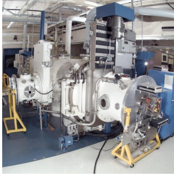
Figure 9. GRC's VF-8 test facility utilized for H64M thruster testing.
